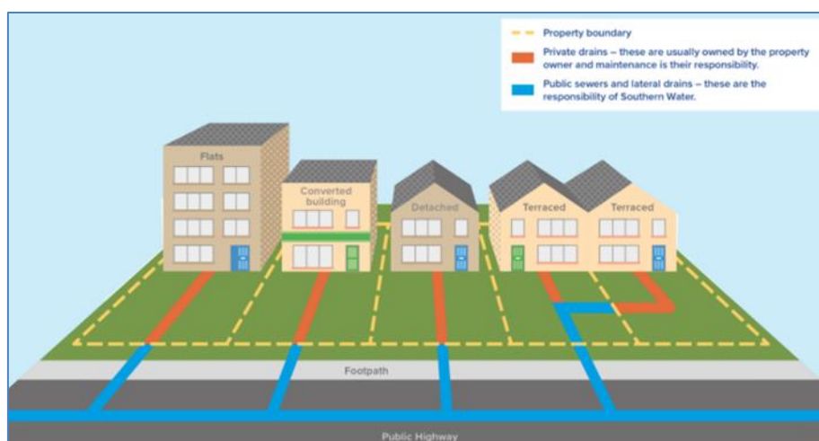
Figure 33 – Drainage Definitions and Responsibilities
