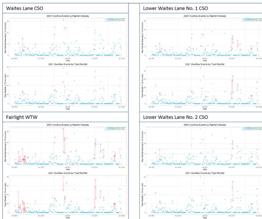
Figure 29 – Storm Overflows - StormHarvester Assessment
