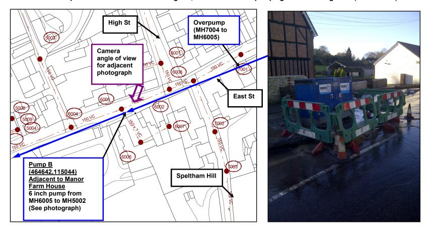
Pump B - Junction of East St and High St, Hambledon - Overpumping and Tankering Sites (Sheet 2 of 8)
